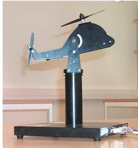
**Figure 1:** The bench-scale 2DOF helicopter from Humusoft.
