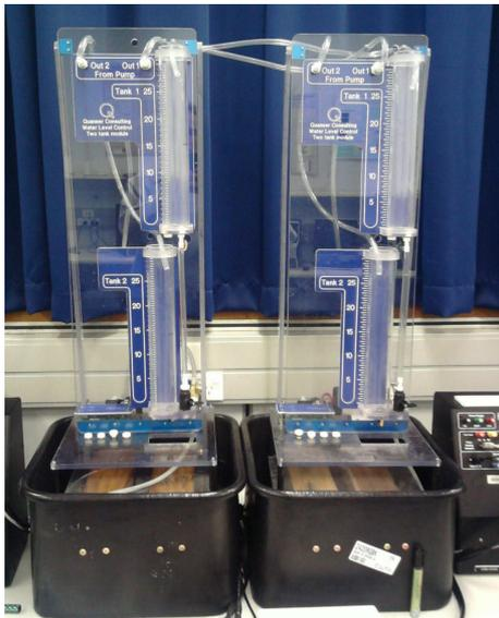
Fig. 4. Two Quanser 2-coupled tanks connected together to form an interacting 4 tank plant.
